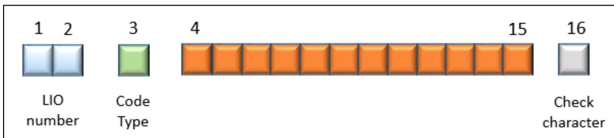
538 539 Figure 1 –Structure of an EIC code
